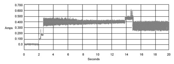
Figure 1 Typical 5V startup and operation current profile
