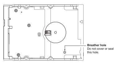
Figure 3 Breather filter hole location
